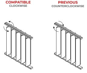
You can choose between feathers that open clockwise or counterclockwise determining the this way determining the opening side of the feathers.
