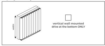
The SUNBREAKER 210 system can be installed in a niche 3or on a substructure. NO BRACKETS FOR FAÇADE MOUNTING!!!
